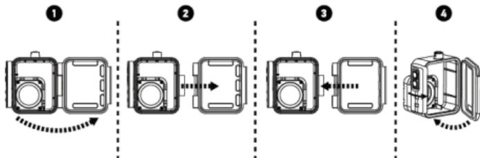
Waterproof Backdoor: Use waterproof backdoor to protect the camera from depths up to 197/60m underwater.
