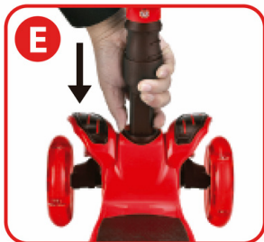
Press red push button. Insert the handlebar with the flat side backwards in scooter hole.
