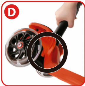
Press Red Switch with one hand and using the other hand to pull handlebar to separate the Handlebar and Scooters body as shown in Figure D.
