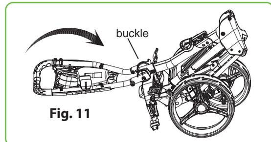
Release the buckle to fold the handle as Fig. 11, then fix the buckle.
