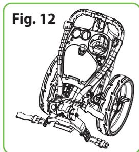
Fixed the frame through elastic rope as Fig. 13. Folding status as Fig. 12. Pick up the trolley using the handle and not the tubing when lifting into car boot etc.
