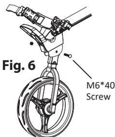
Remove the M6\*40 screw and M6 nut from the front wheel fork as Fig. 6, then assemble the front wheel on the steel piece of lower bag bracket and fixed it by screw and nut, completely assembly as Fig. 7.
