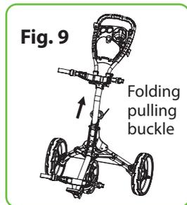
Pull the folding pulling buckle and press the handle to fold the trolley as Fig. 9 & 10.
