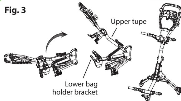
Hold the upper tube and lower bracket to open the frame as Fig. 3
