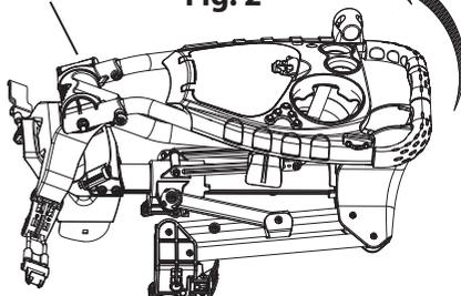
Release the handle buckle to fully extend the handle frame then lock the locking buckle as Fig. 2.
