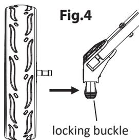
Release the wheel locking buckle, insert the wheel axel into the wheel holder completely and then tighten the locking buckle.
