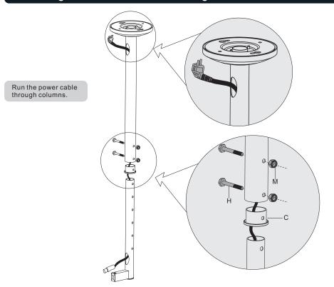
Insert plastic bushing and inner column into the outer column and fix them at the desired height using the correct combination of screw and nut.
