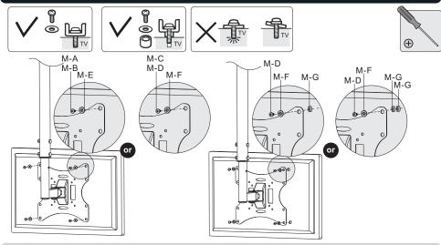
**Note:** Choose the appropriate screws, washers and spacers (if necessary) according to the type of screen. Lift the display and match the holes on your display with the holes on the mount. Secure your display to the mount by tightening screws.
