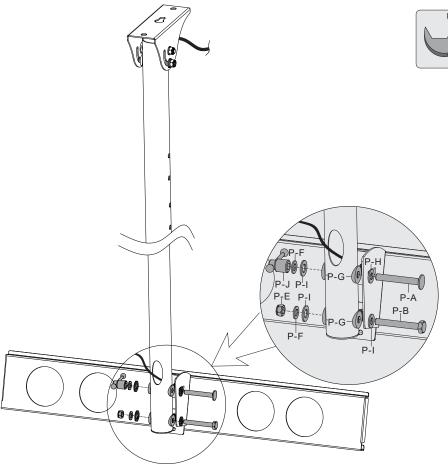
Assemble the universal plate and bottom pipe with connect plate. Using correct combination of screws, washers, nuts and iron knob.
