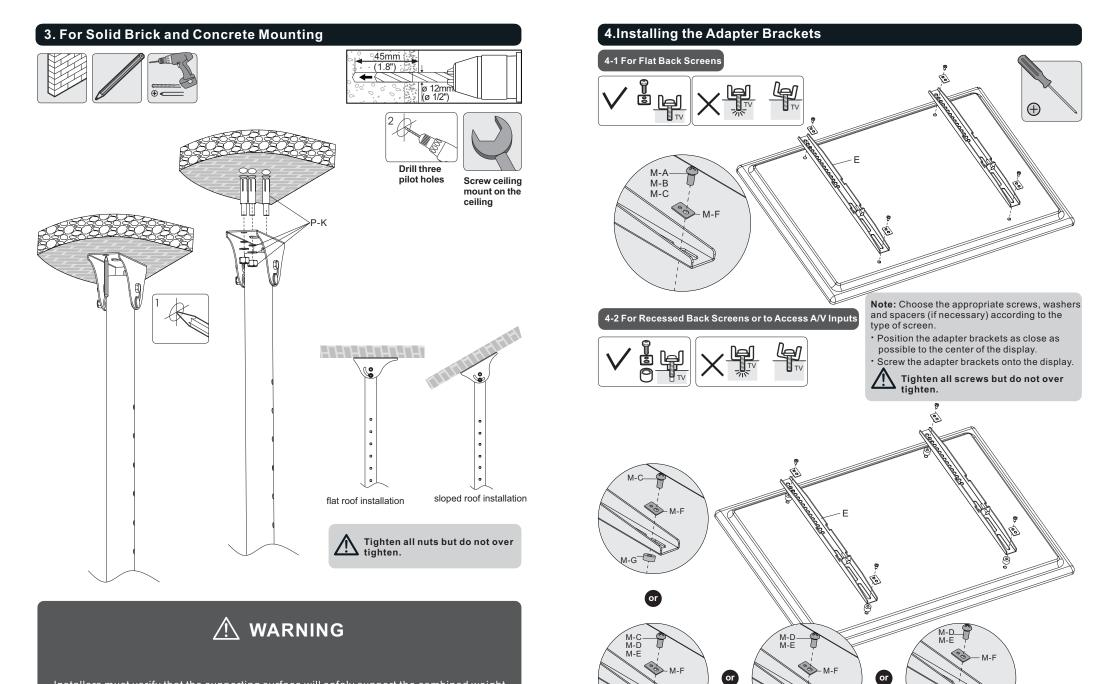
Installers must verify that the supporting surface will safely support the combined weight of the equipment and all attached hardware and components.
