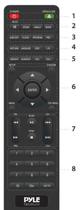
1. **Standby/Power on/off switch:** Press to open/close the unit power. In this mode, he unit is still consuming a small amount of power.
