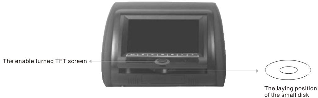
Notice: Please carefully turns on the display monitor when vehicles start , please to close the display monitor after puts well the small dish as soon as possible, in order to avoid damages to the display monitor.
