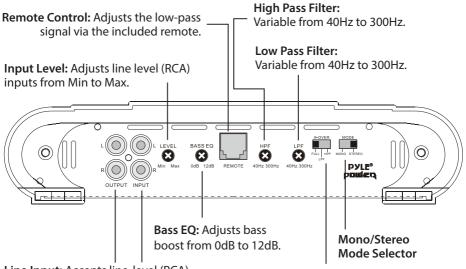
**Line Input:** Accepts line-level (RCA) inputs from 0.2 to 5 volts.
