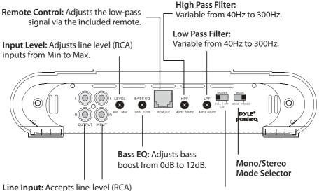
inputs from 0.2 to 5 volts.
