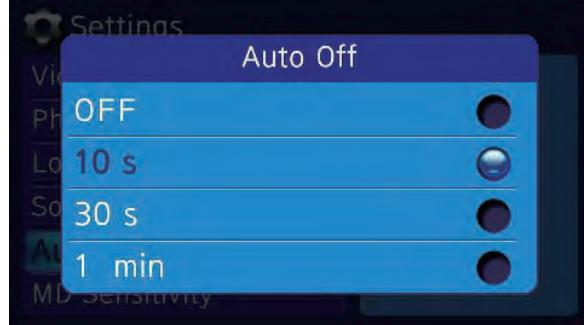
Set auto power off time (10 s, 30 s, 1 minute) when external power source is unplugged.
