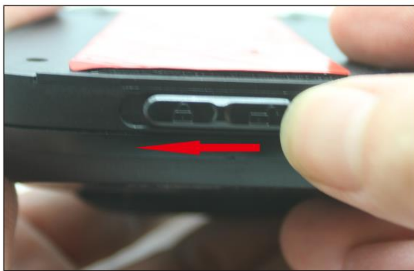
3. Push the locking bar towards the left
