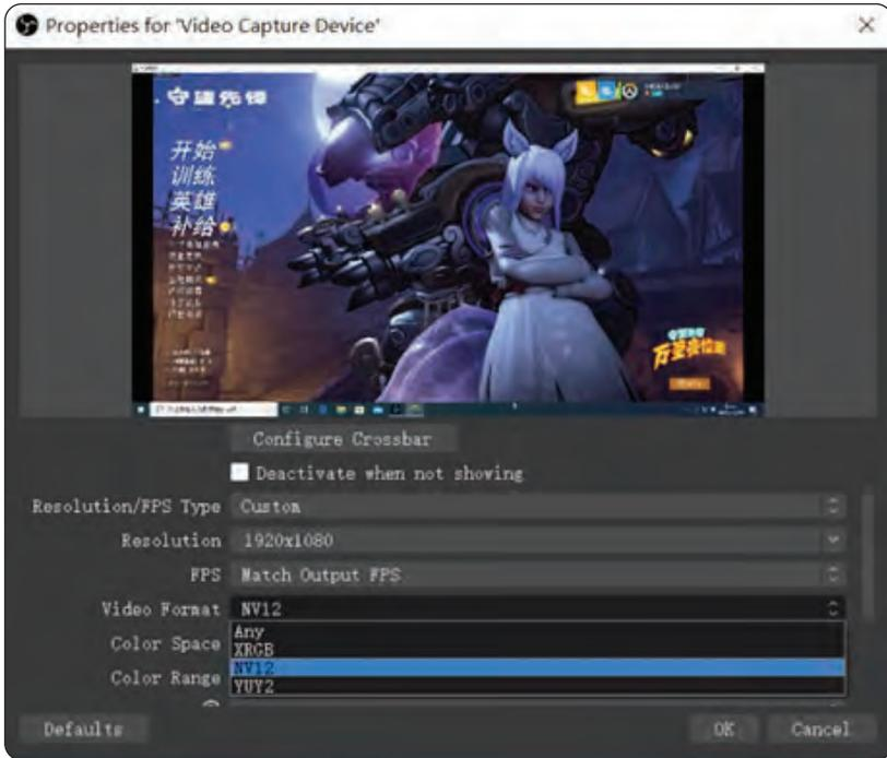
The video format options depend on resolution, the max FPS depends on both resolution and video format:
