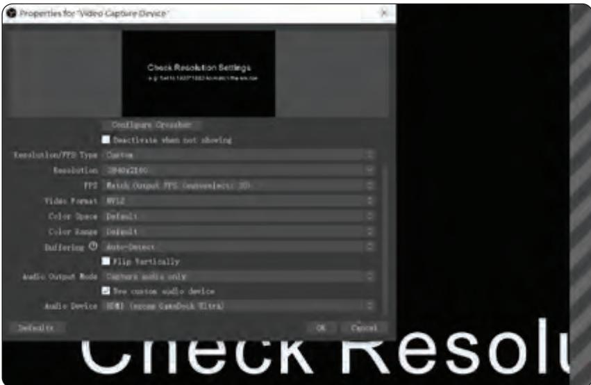
Set to 4k while input is not. Set to lower resolution to match the source.
