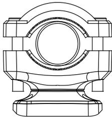
For diameters ranging from 0.83 to 1.57 inches, use the 35mm screws.
