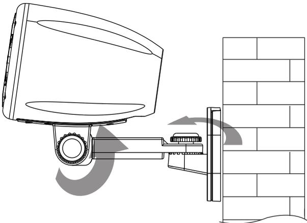
The front bracket can be rotated up and down, and the rear support can be rotated around.
