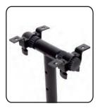
Slide the metal mounting clamps onto both ends of the extension arm. Each side is fitted with rubber grips that the clamps use for holding support. Be sure as to, at least partially, slide the metal mounting clamps to lay over the rubber grips. Use the dual clamp-style knobs on both sides on each of the mounting clamps to secure the angle and placement of the device resting plate.
