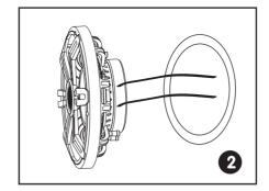
Connect the speaker wires to the speaker.
