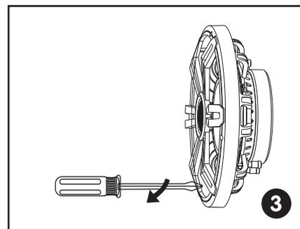
Screw down each of the four Phillips head screws. The locking tabs will swivel into place and secure the unit to the rear surface of the drywall. Put in the strips of adhesive to secure the grille.
