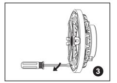
Screw down each of the four Phillips head screws. The locking tabs will swivel into place and secure the unit to the rear surface of the drywall. Put in the strips of adhesive to secure the grille.
