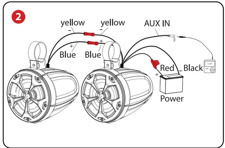
**Step 7:** Connected two speakers by RGB connect wire, see the drawing in below
