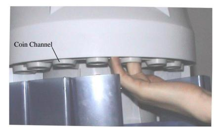
If the machine isn't put on the **horizontal** or it **shakes** too much when it's working, sometimes a coin will falls in a smaller Coin Channel by error and then it will cause a jam. To settle this error, please push the coins in the jam-packed channel with the finger and then let them down from the gap between two coin channels just as the picture above.
