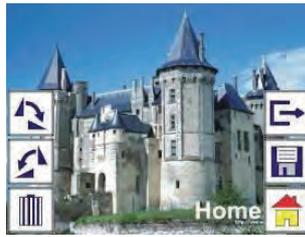
Select Home icon with LEFT/RIGHT button, then press OK button or press MENU button on top of the device anytime to return to main menu
