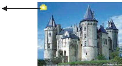
Once entered capture mode, there will be an indicator on the left top corner to indicate it is in live view mode. User can also press OK button, then press **LEFT/RIGHT** button to adjust EV value, press **SCAN** button again to confirm and back to live view mode.
