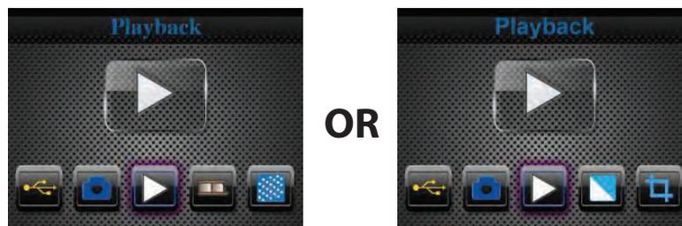
Press LEFT/RIGHT button to playback mode when power on the device or access the main menu by Home icon/MENU button anytime. Press OK button to confirm the selection.
