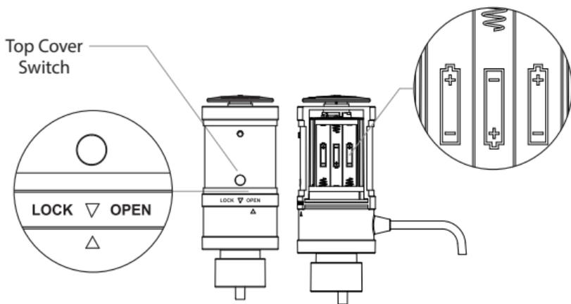
Remove the Top Cover from the Electronic Body Assembly by pressing the Top Cover Switch and turn the cover to the right (counterclockwise) and pull the cover up and off the Electronic Body Assembly to expose the battery compartment
