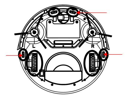
Slightly wipe all sensors and wheels, as marked in above figure, with soft cloth or tool.
