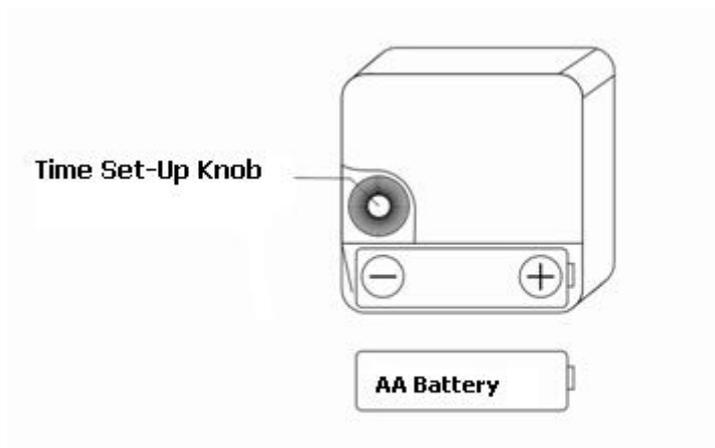
3. Adjust the minute hand by using the Time Setting knob. Never turn the hour hand to set the time; it will turn automatically with the minute hand. Turn the Time Setting knob or move the minute hand (**AFTER** the batteries have been installed) so that the hands rotate clockwise
