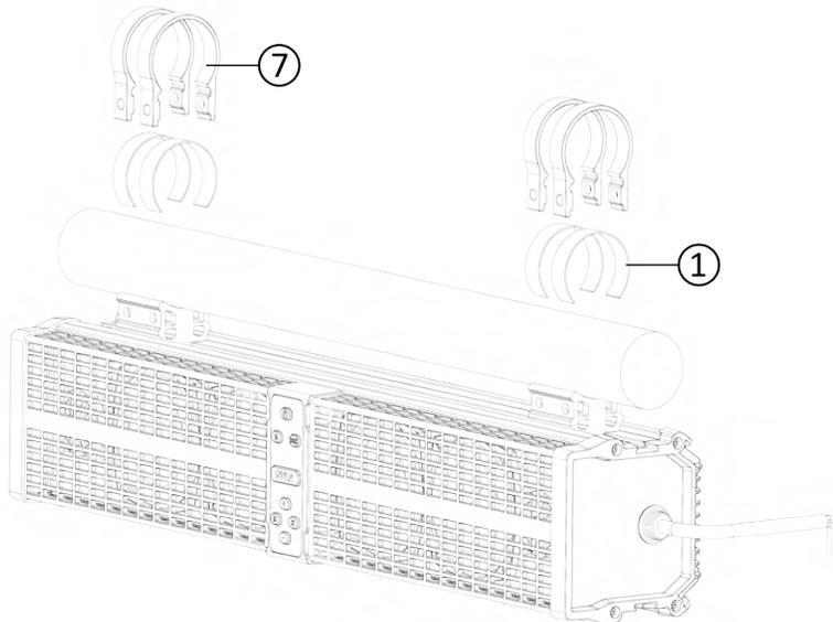
4. Installing on the cage bar of 1.5" to 2.0". Wrap the rubber strip on the cage bar to prevent being scratched. And then, press the aluminum rings on the rubber strip. The screw mounting holes of the aluminum ring are aligned with the base.
