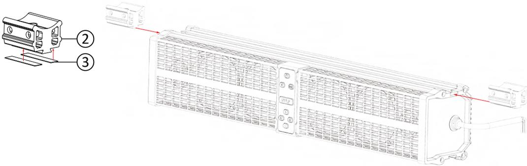
1. Stick the 45X10X0.5mm non-slip rubber strips (2 pieces) on the bottom of the clamps, then insert them into the slider.
