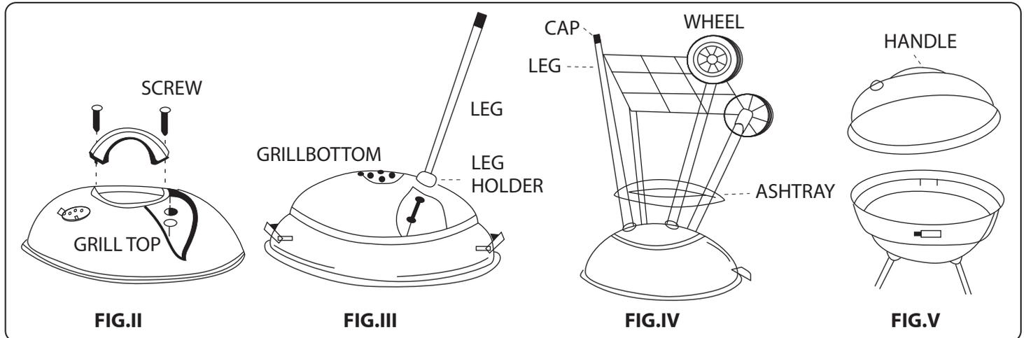
1. Install the curved phenolic handle (14) and lid hanger bracket (15) to the grill top (1), using two screws (13), nut (16).
