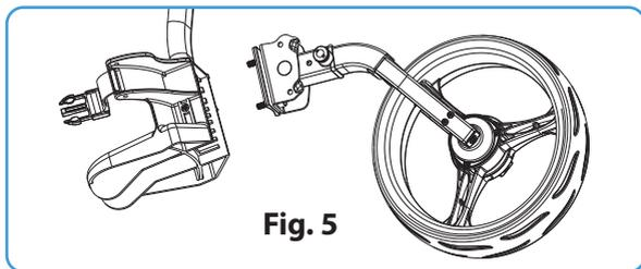
Take out the fixed steel piece from the front wheel package, then going the screws through the holes and keep the "up" toward upper as Fig. 5.
