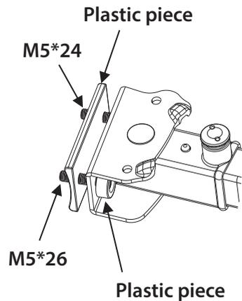
Completely unfolding and assembly as Fig. 6.
