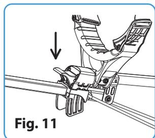
Press the red button and adjust the slide lock to required handle height as Fig. 11
