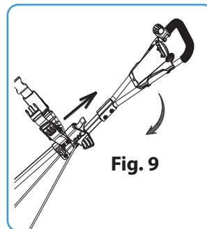
Move the slide lock up to release the handle as Fig. 9
