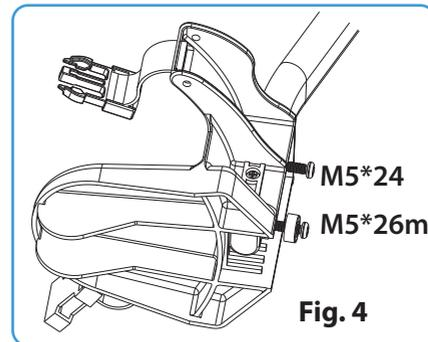
Remove the screws and Plastic piece as Fig. 4.
