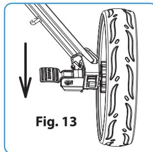
When the red brake pedal is engaged, it should work with a gentle downward pressure; If it does not, slightly move the wheels until the braking pin can seat easily. The mechanism should last for years if treated good. Step on the brake pad to activate and pull off to deactivate the brake as Fig. 13
