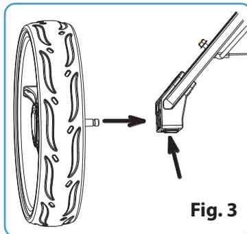
Press the red button on the wheel lock mechanism to assembly rear wheel as Fig. 3
