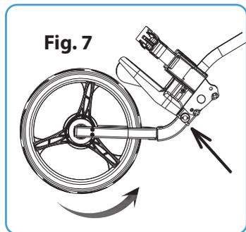
Press the red button to release the front wheel, then fold until the pin inserts in the hole as Fig. 7 and 8.
