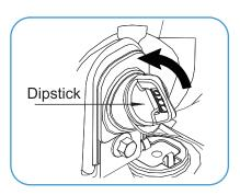
Reinstall dipstick into hole; rest on oil fill neck. **DO NOT** thread cap into hole. Remove the dipstick again and check oil level. Level should be between the upper and lower limit.
