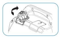
3. Turn the ON/RUN switch to the "RUN" position.
