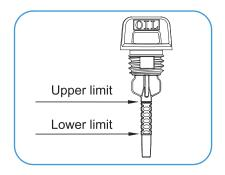
Reinstall and fully tighten the dipstick.
