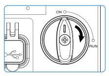
4. Turn the energy saving switch to the "**ON**" position.
