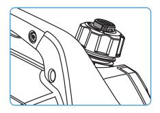
The fuel tank cap is equipped with the ventilation knob to prevent leakage of fuel. The ventilation knob must in "ON" position when operating generator set. Because this makes the fuel be injected to the carburetor and drive the engine. To avoid fuel leakage, turn it in "OFF" position when carrying or not use the generator set.
