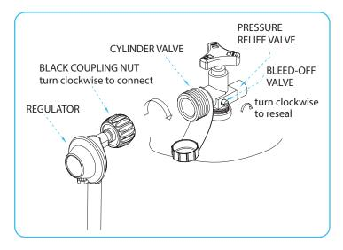
Turn the cylinder valve on the tank clockwise to close the propane tank. Attach the preassembled regulator from the Body to the cylinder valve by turning the regulator coupling nut clockwise. Make sure it is fastened securely and tighten connections by hand only.
