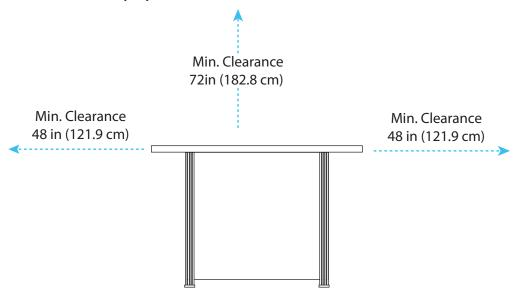
Combustible materials should not be within 72 inches of the top of the unit, or within 48 inches around the entire unit.
