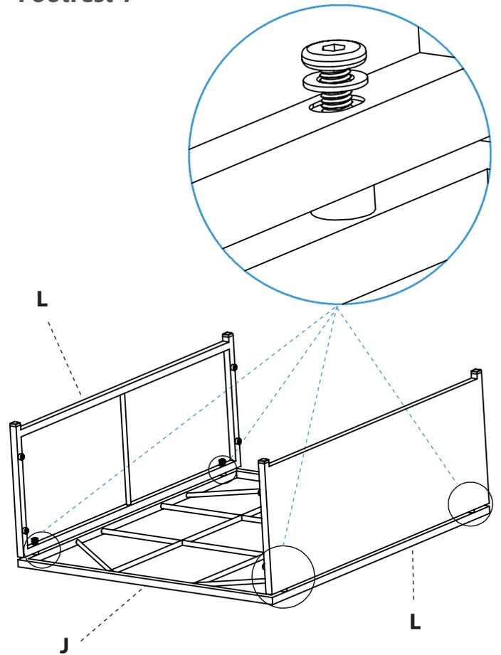
Finally, tighten all the screws!
