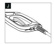
Insert the high pressure hose tightly in to coupling on the appliance, it will lock in audibly.
